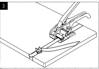
Press the handle to lift the gripper leg so the strap can be put under the gripper
