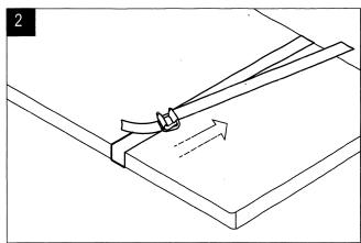
Put strap and buckle around package and manually pull to tighten the strap.
