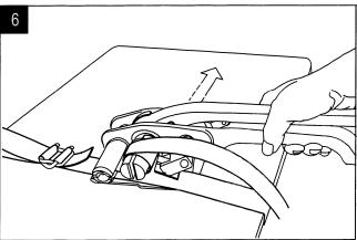
Depress the handle to cut the strap. Pivot tensioner away from the strap
