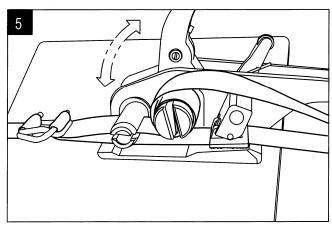
Hold the tool and strap with your left hand and move the handle forward and backward until the strap is tensioned
