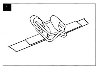
Thread the strap through the buckle as shown. Keep legs of buckle pointing to the right.
