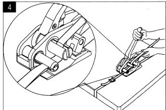
Slide the upper strap through the slot of cutter and windlass
