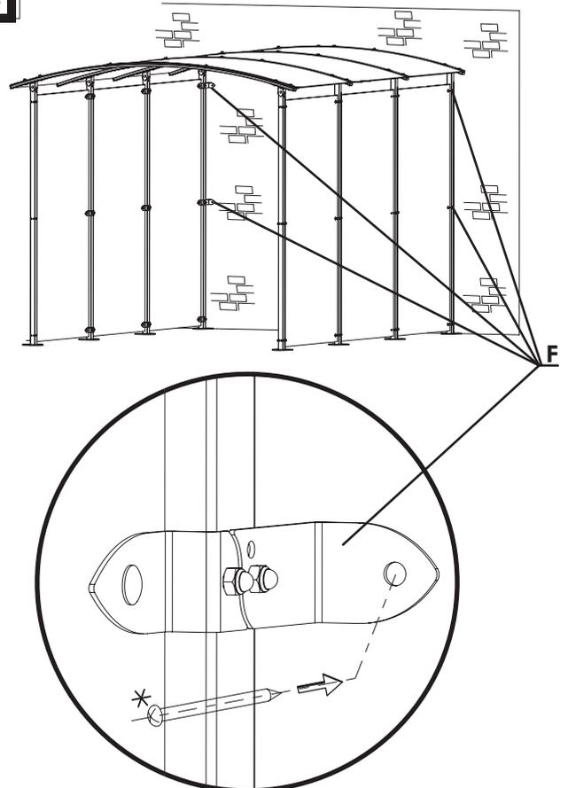
\* Fixations au sol non fournies / Assembly on the ground not provided
