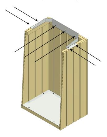
4 Get the lid assembly and attach to the back side of the rear panel with screws provided.
