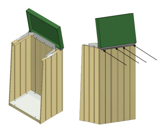
5 Hook the front panel on to the brackets fitted on the right and left side panels.
