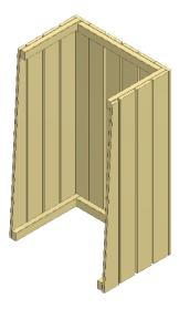
NOTE: The sloped board of the side panels should be facing forwards.
